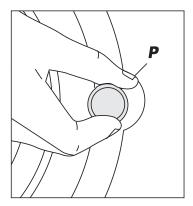
Plastic plugs, supplied inside the protective bag and designated as "P", should be placed in the safety bolt holes according to the direction shown
